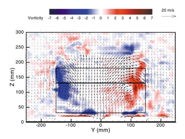
The figure shows vorticity contours and corresponding interpolated velocity vectors for a hatchback car measured in a plane normal to the mean flow. The data was collected at a wake survey plane 2.5 car heights behind the 'hatch'. The measurements show the instantaneous wake is not symmetric and is dominated by two time-dependent, counter rotating, primary, trailing vortices. The data was processed using custom software designed to compensate for through sheet motion and viewing angle.
